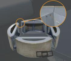
Place the 4 pieces together. Line up the holes on each piece with the corresponding holes and drill in the self tapping screws. Do this for all 8
