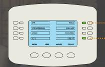
This is Firegear's Home/Pool Automation Transmitter. It allows you to operate your Firegear TFS product from the same controller you're used to using your pool system. It's important to note that even though you are using the HAT, you can still use your original remote that came with your TFS unit.
